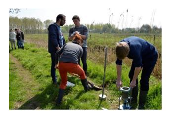
Different issues were proposed: measurement of Radon in soil air with Lucas cells, gamma spectrometry on Demerbroeken soil samples and comparison with non contaminated soil, in situ gamma spectrometry allowing to compare the situation in Demerbroeken and Brussels, assessment of Radon in dwelling air after trapping it with charcoal canister. We were also interested in the measurement of natural radioactivity
